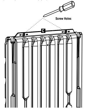
Snap Repeat Left Side (C) into the back position of Repeat Floor (B).
